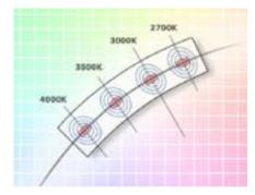
Corrected Cold Phosphor Technology® Xicato XSM modules perform to less than a 2 step MacAdam Ellipse as illustrated.
