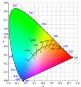
A CIE x,y chromaticity space diagram illustrates where the black body locus defines white light. It also shows black-body light sources of various temperatures and lines of constant correlated colour temperature.
